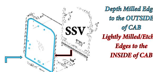
Depth Milled Edges to the OUTSIDE Lightly Milled/Etched
