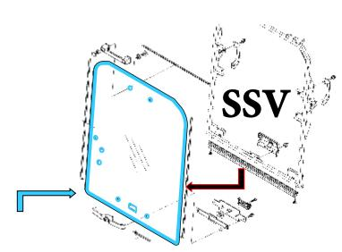
Depth Milled Edges to the OUTSIDE of CAB Lightly Milled/Etched Edges to the **INSIDE of CAB**
